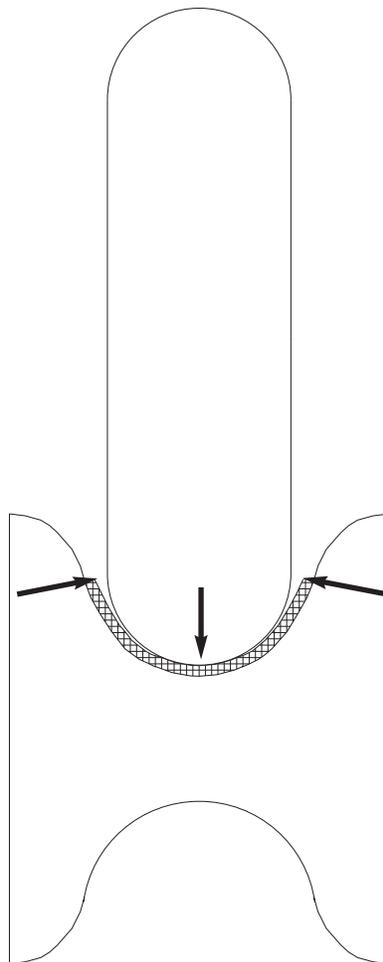
*Fig. 2—Forming material thinner than the design gauge results in a larger radius, as shown here. Material not contained by the rolls bends at the points indicated.*
