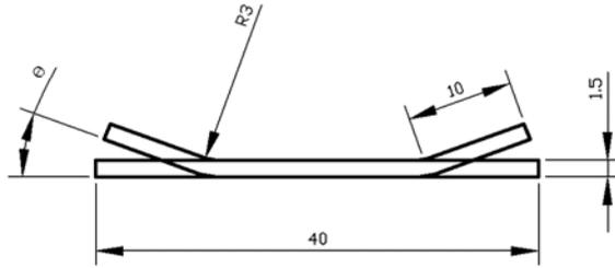
**Figure 2.** The geometry of an undeformed strip and a strip that has been formed.
