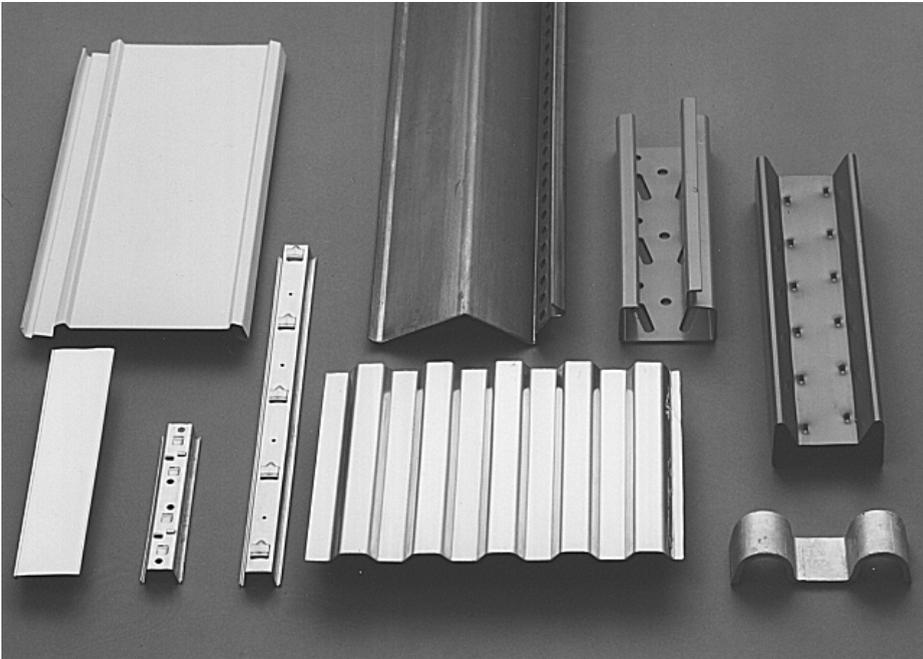
**Figure 1.** CRF products can be find in many applications as vehicles, buildings, domestic appliances etc.
