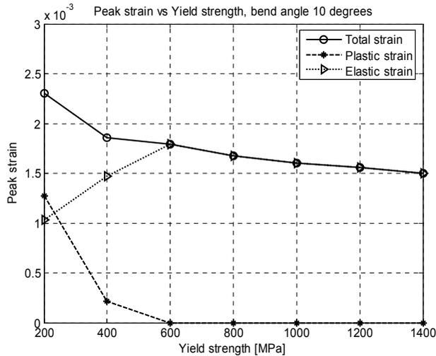
**Figure 4.** When the yield strength increases the longitudinal peak membrane strain will decrease. When the plastic strain goes to zero the total strain will flatten out and the strain is purely elastic.
