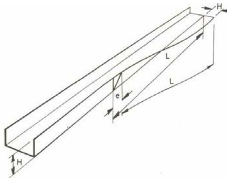
**Figure 3.** The material in the flange will travel a longer distance than the material in the bending zone. That difference will cause a strain ( $e$ ) in the flange. In the figure are ( $H$ ) the flange length, ( $L$ ) the deformation length and ( $e$ ) the strain in the flange, [1].
