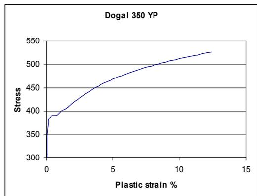
**Figure 4.** Stress - strain curve for Dogal 350 YP.
