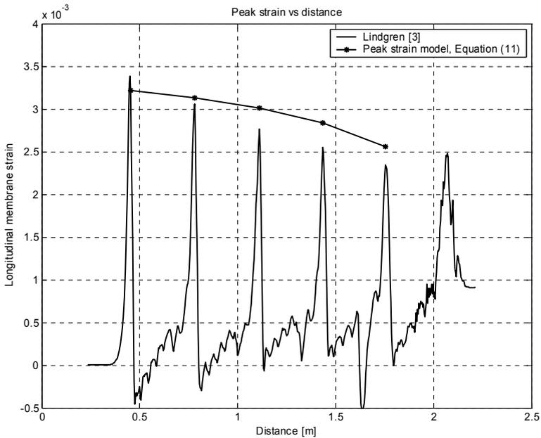
**Figure 9.** The model Equation (11) is compared with the simulation result Lindgren [3]. The model predicts decreasing peak strain well when constant forming increment is used. In this case is the constant forming increment  $15^\circ$ . For the  $90^\circ$  forming step is the Equation (11) not valid.
