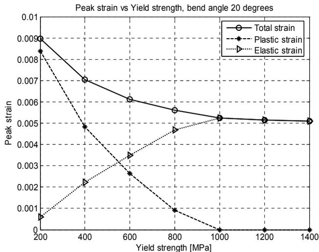
**Figure 5.** The behaviour for the longitudinal peak membrane strain is similar as for the case with a forming step of  $10^\circ$ . But now is the curve for the elastic and plastic longitudinal peak membrane strain displaced to a higher level of yield strength.
