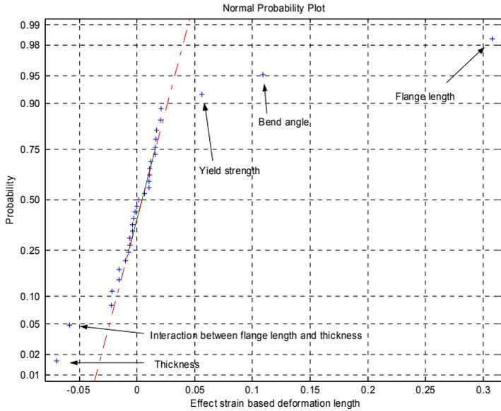
**Figure 4.** Normal probability plot for the deformation length.
