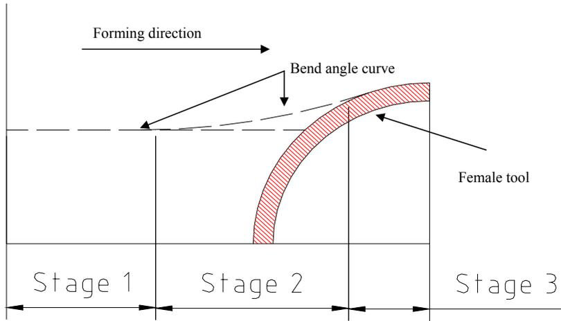
**Figure 10.** The bend angle is divided in to three stages, stage one where the angle does not change, stage two where the angle changes but the strip is not in contact with the tool and stage three where the strip is contact with the tool.
