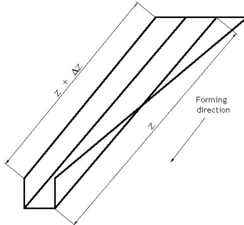
**Figure 1.** The material will travel a longer distance  $\Delta z$  in the flange than in the bending zone.
