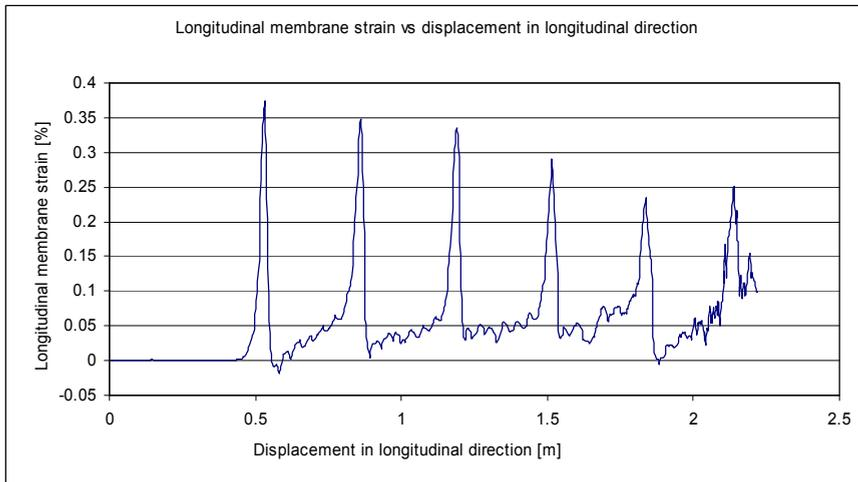
**Figure 5.** The longitudinal membrane elastic - plastic strain in the edge of the strip in six forming stands. Constant forming steps are used (15 - 30 - 45 - 60 - 75 - 90).
