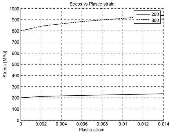
**Figure 3.** Stress – strain curve for the material hardening.
