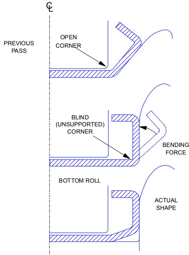
Figure 4.2.7.1-3 Possible additional bendline at unsupported section
