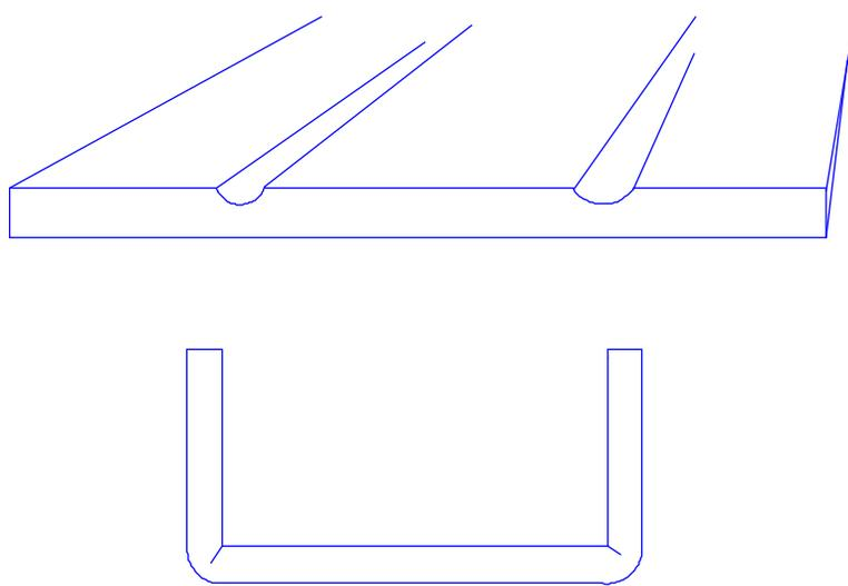
Figure 4.2.7.1-1 Grooving strip to form sharp corners
